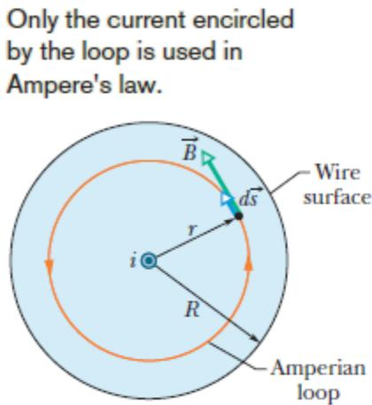
**Fig. 14** Using Ampere's law to find the magnetic field that a current  $i$  produces inside a long straight wire of circular cross section. The current is uniformly distributed over the cross section of the wire and emerges from the page. An Amperian loop is drawn inside the wire.
