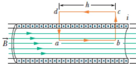
Fig. 19 Application of Ampere’s law to a section of a long ideal solenoid carrying a current  $i$ .
