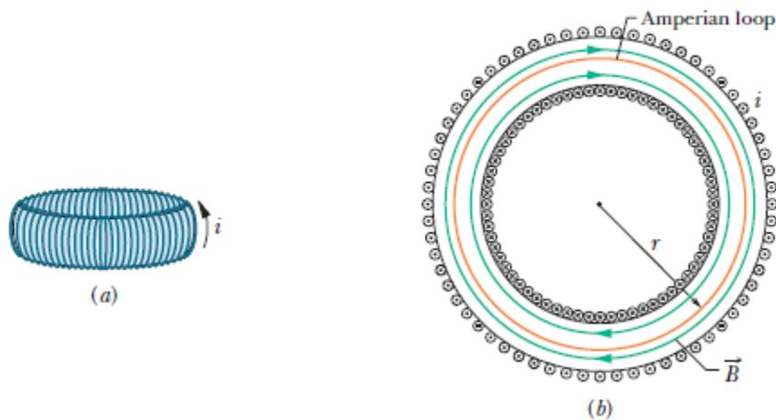
Fig. 20 (a) A toroid carrying a current  $i$ . (b) A horizontal cross section of the toroid. The interior magnetic field (inside the bracelet-shaped tube) can be found by applying Ampere's law with the Amperian loop shown.
