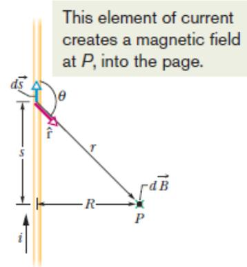
**Fig. 29-5** Calculating the magnetic field produced by a current  $i$  in a long straight wire. The field  $d\vec{B}$  at  $P$  associated with the current-length element  $i ds$  is directed into the page, as shown.
