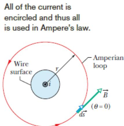
**Fig. 13** Using Ampere's law to find the magnetic field that a current  $i$  produces outside a long straight wire of circular cross section. The Amperian loop is a concentric circle that lies outside the wire.
