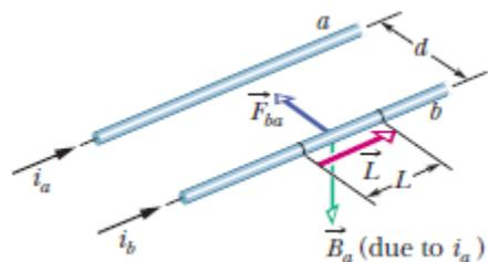
Two parallel wires carrying currents in the same direction attract each other.  $B_a$  is the magnetic field at wire  $b$  produced by the current in wire  $a$ .  $F_{ba}$  is the resulting force acting on wire  $b$  because it carries current in  $B_a$ .
